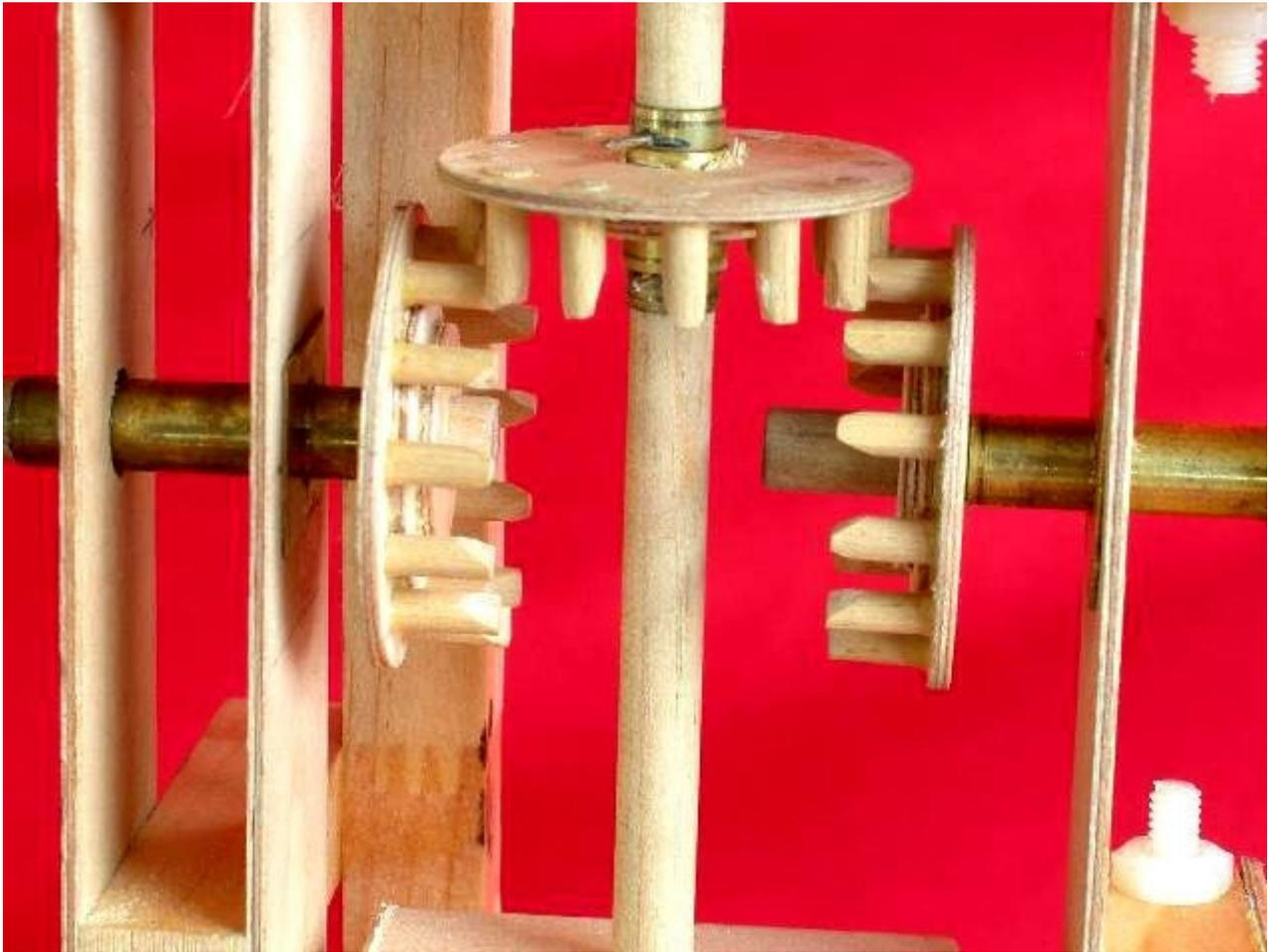
If the left gear turns in a direction, the gear on the right-hand side will turn in the opposite direction.
